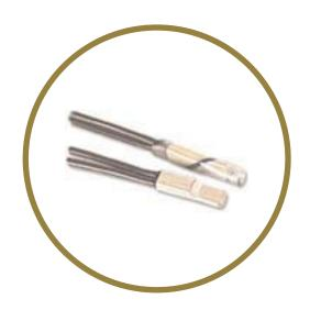
In addition to being small and lightweight, the unit is both temperature and current sensitive. Since the 9700 is sealed to withstand varnish dipping, it can be mounted directly in windings where it can best sense the true temperature of the electrical equipment. As a result, over-temperature protection is assured.
