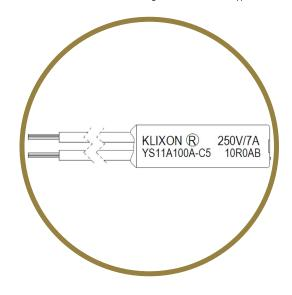
The YS11 can be used for on-winding and outside of resin packed motors by clamping or insertion. Since the YS11 has a plastic case, it does not need to be insulated from metal part of the motor.
